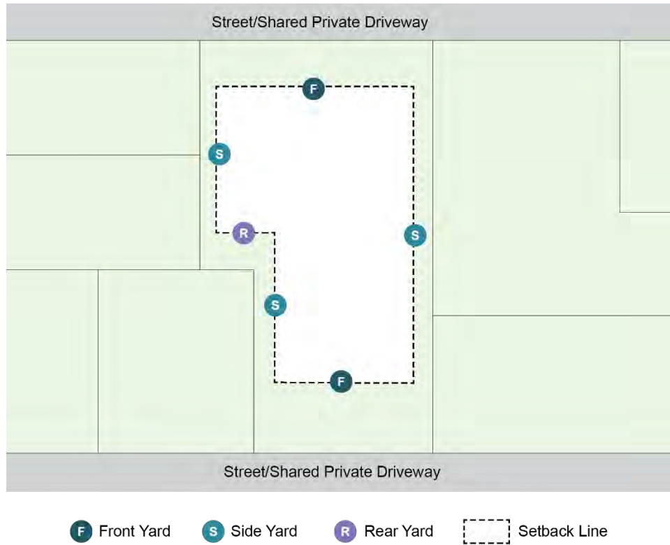
Figure 16.4.11-2: Typical Location of Yards and Setback Lines on a Double Frontage Lot
