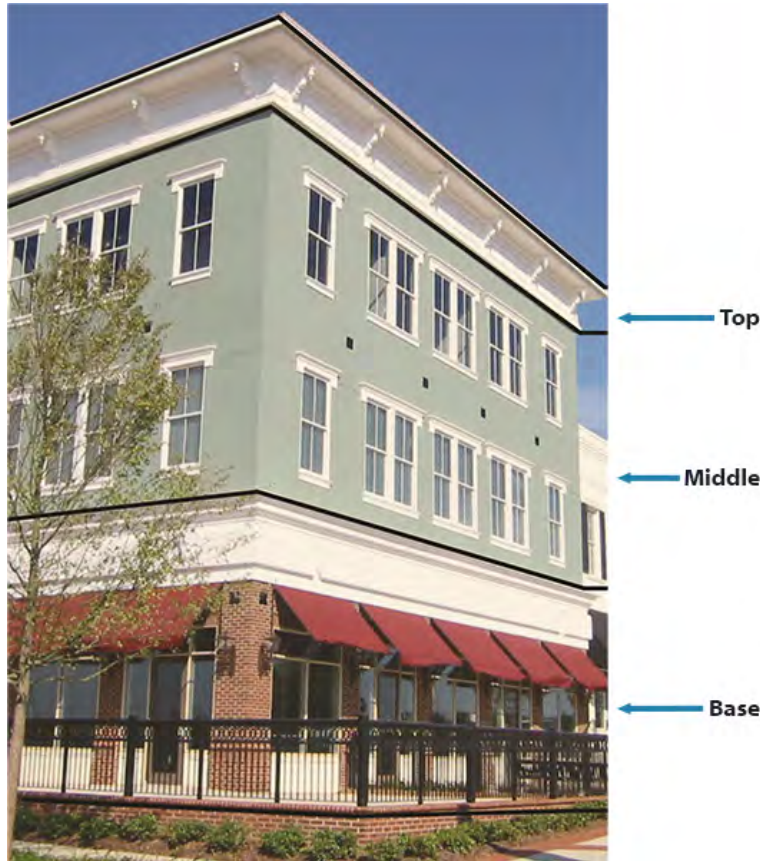
Figure 2.3.6-2: Building Façade Elements
